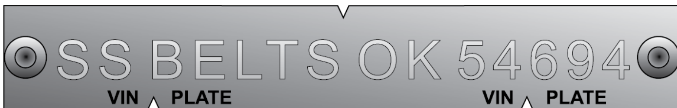
Figure 7-5-4. Example of plate fitted to a vehicle that may retain single-sensitive front seatbelts
